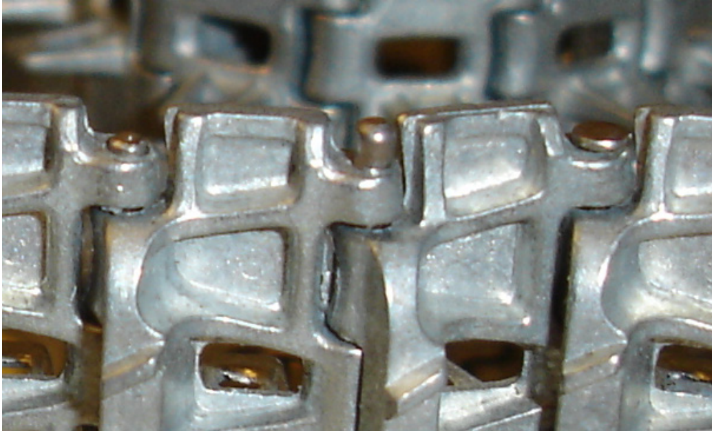
Left to right; new track pin fully inserted, new track pin awaiting the hammer and punch, and old track pin.
