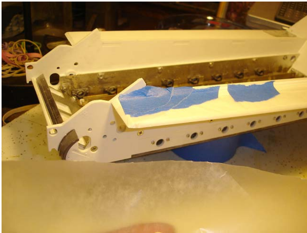
Wax paper is wrapped over the panniers to seal them from the filler and glazing putty.
