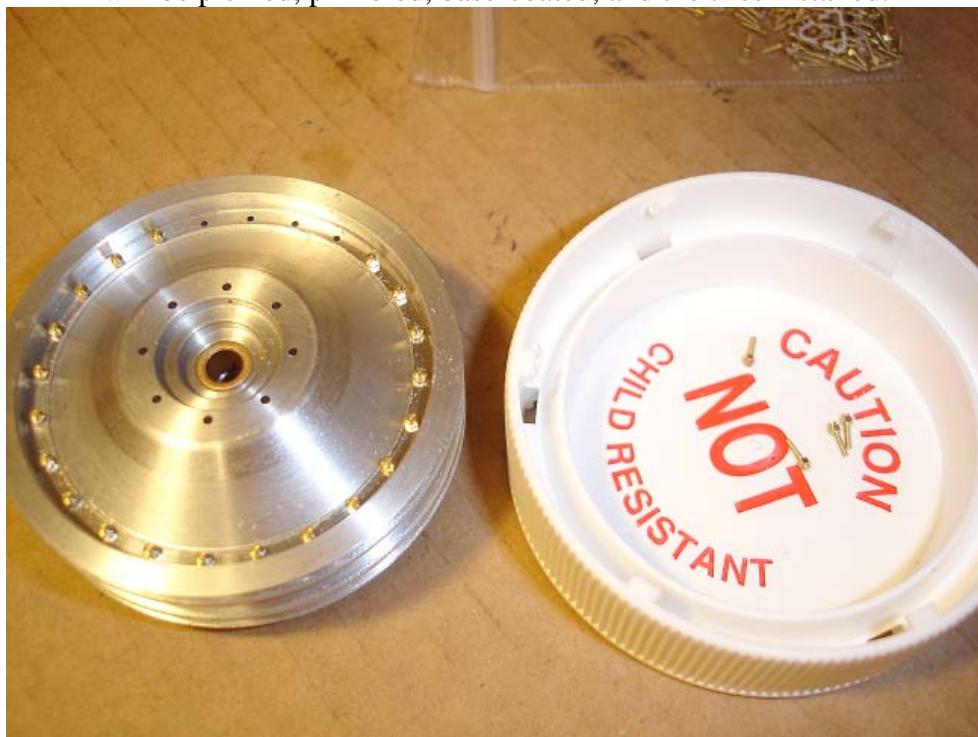
The 24 outer bolts are being installed, 8 larger ones will go in the inside 8, and 8 more on the hub cover
