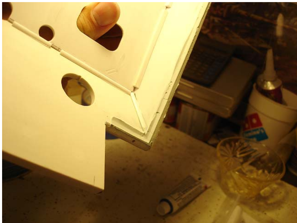
Filler has created a seating lip for the panniers in the upper hull.
