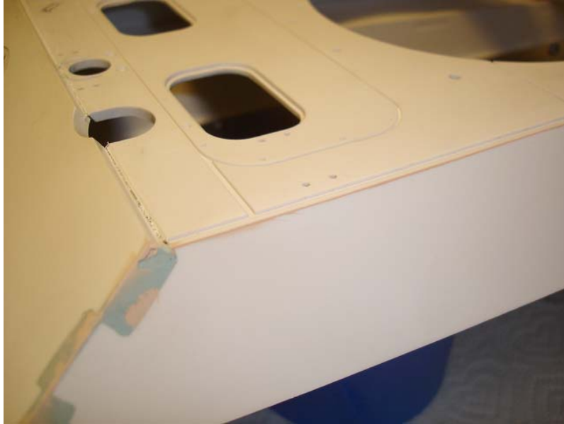
After wet sanding, clean joints are left. The area on the upper left will have to be slightly cleaned out and an additional coat applied, then wet sanded.
