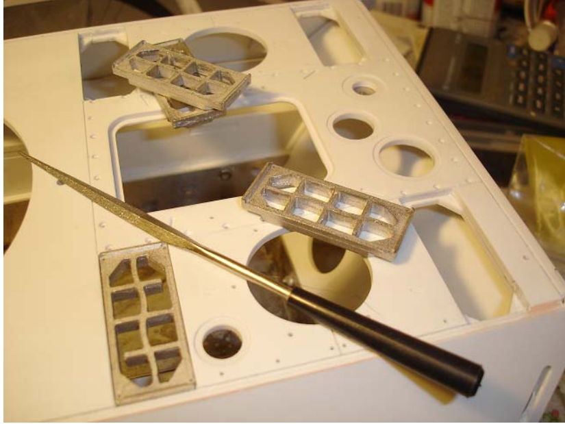
Cleaning up the radiator air cooling induction grates.
