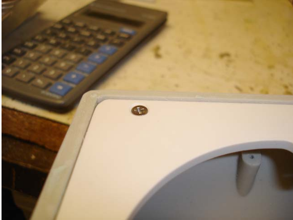
Screws heads installed below the surface of the plate.
