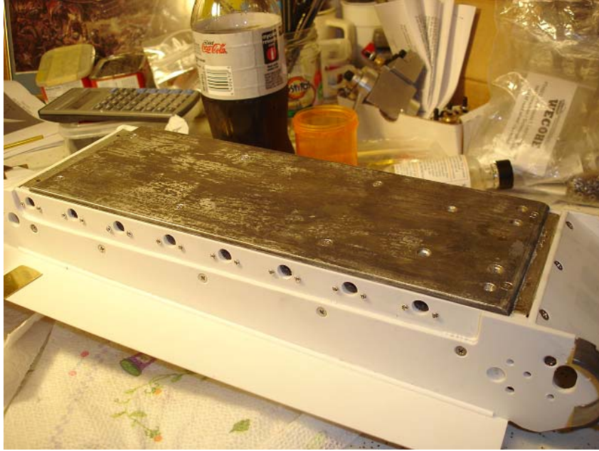
Here is the strengthening plate after pickling and being mounted to the lower hull.
