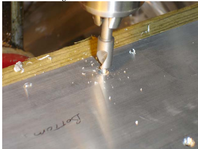
These flathead screws required a countersink with angles of 90°. My toolbox had two countersinks and neither was a 90°, so I had to get yet another.
