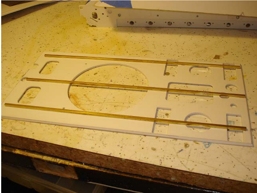
The bottom of the upper hull deck with brass tubing positioned to keep bending of the deck at a minimum.
