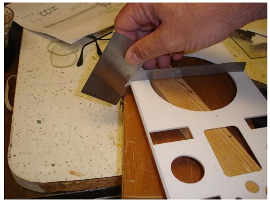
Here's a picture of the metal angle maker with an angle of 60° selected. To tune-in the final angle on the plastic, you can drag the angle maker along the angle made and it will remove the high spots. On the leading edge of the angle maker you can see the desired plastic being removed and leaving an incredibly tight and accurate edge.
