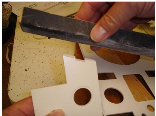
Not shown in this photo is the angle maker. I set the angle maker to the desired angle, visually related that angle to the edge and piece, and started sanding. It's far easier using a larger block when doing these angles, as they won't waiver as much as a smaller sanding
