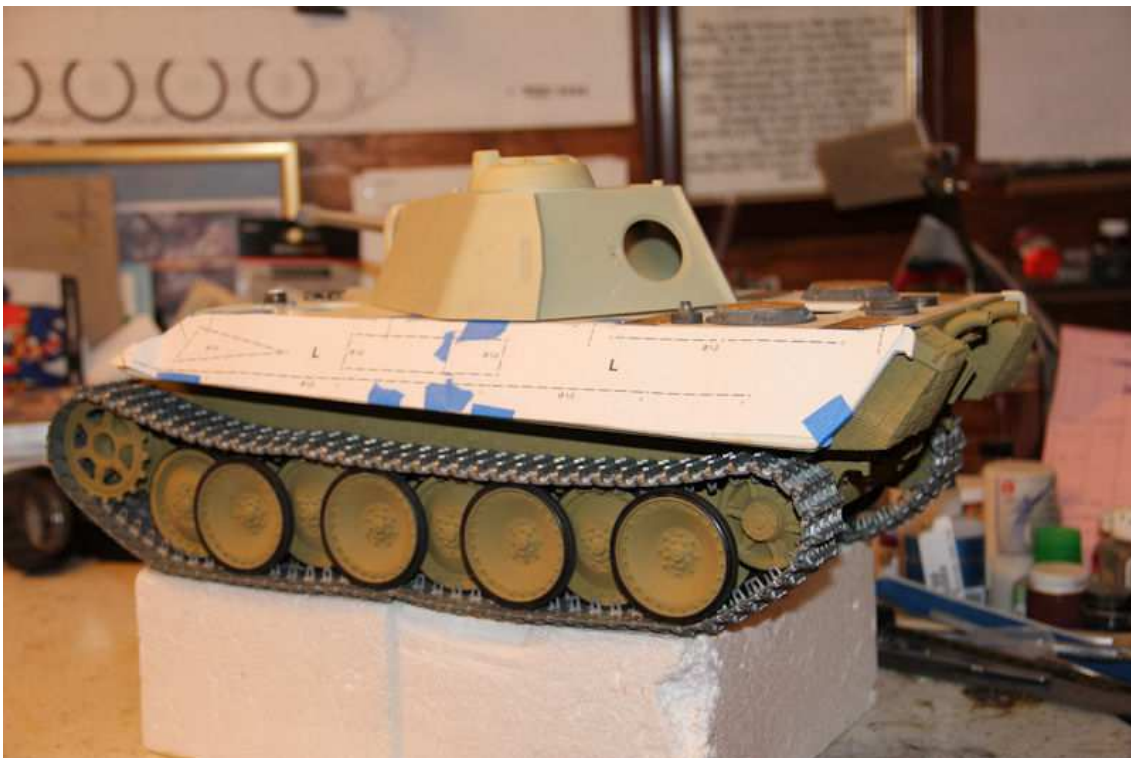
Attached to the side here is the drill-guide. This is the next order of business for this tank; completion of all the components that attach to the sides; most are photo-etch.
