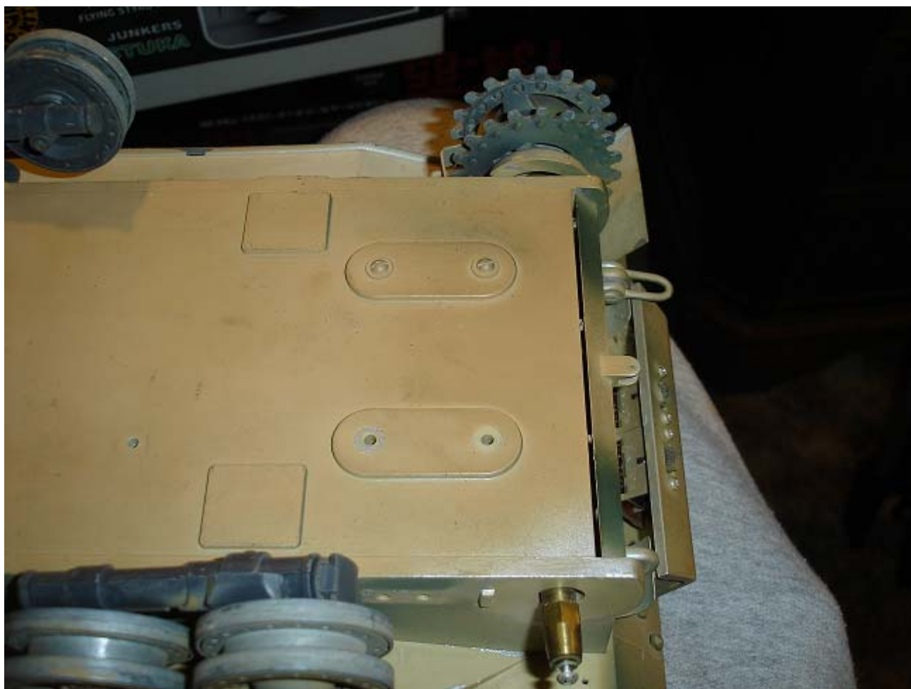
Since this tank was never run, no hull fracturing had occurred.
