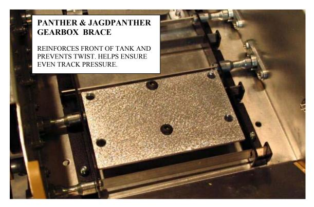
The above item includes three-piece gearbox brace, two socket head screws, large 4mm screws for gearbox mounting, hex key for socket head screws, and instructions.
