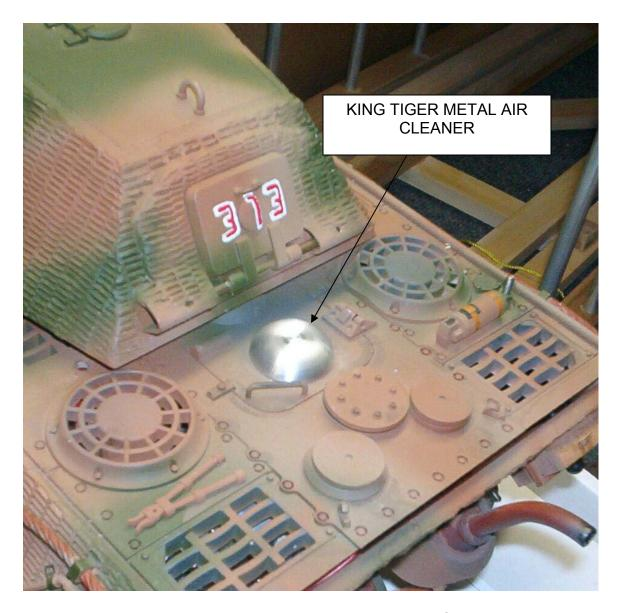
The metal air cleaner is an aluminum replacement for the standard plastic air cleaner. Its heavier design will allow faster removal, acting as a wing-nut when you spin it. Can also act as the cosmetic replacement of the air cleaner on non-Full Option King Tigers and other projects that require this style of air cleaner.
