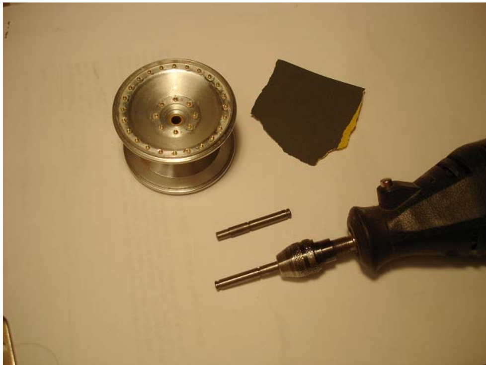
Polishing each wheel shaft to fit.
