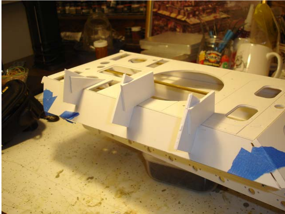
Here temporary angles are positioned while the side hull pieces are being glued.
