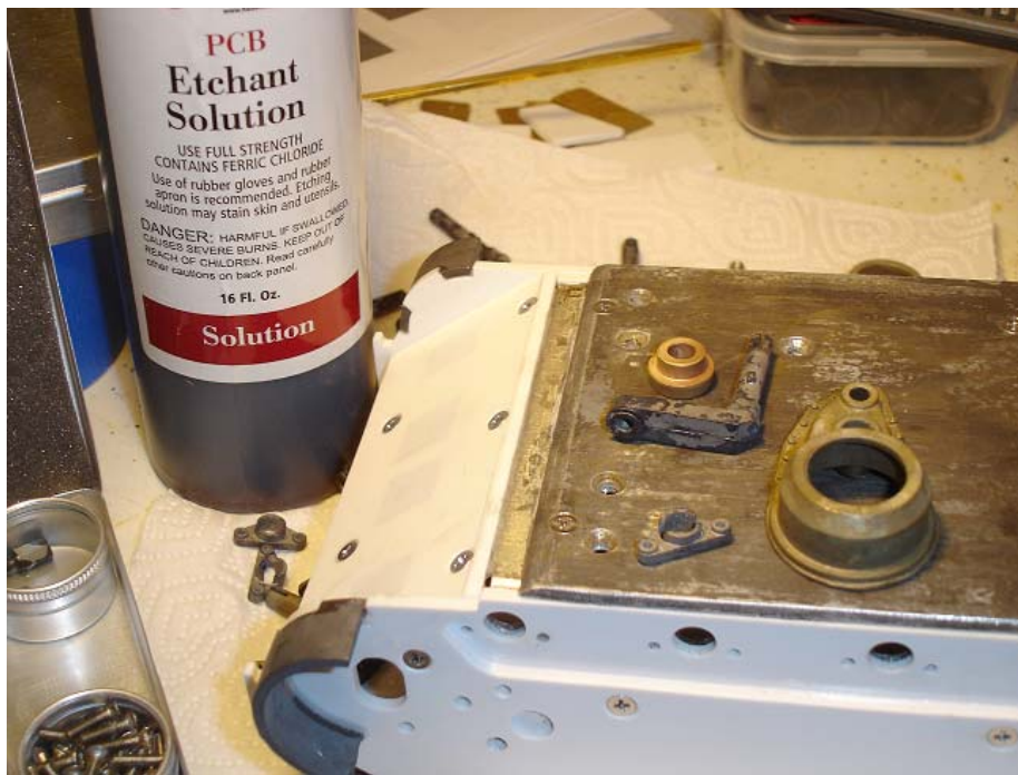
In this photo, seven different metals are shown to be pickled. The swing arm (made of zinc) and the lower drive housing guard (made of white metal) seen mounted on the forward end of the hull were immersed for 1-2 seconds.
