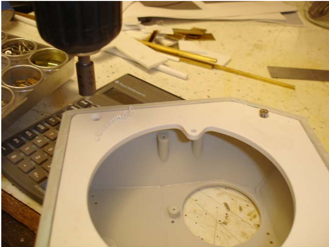
The inside rim of the lower plate has been cut to conform to the inner turret sides, and the screws are being installed.
