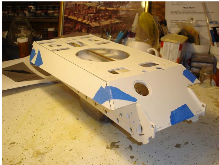
Proof-fitment of the pieces to be assembled, noting any problem issues.
