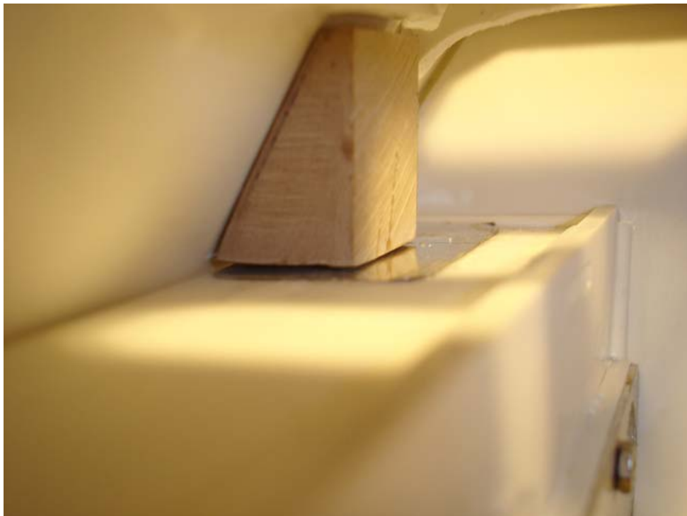
The foam fitted in place flush against both the hull side and seated on the tin plate.
