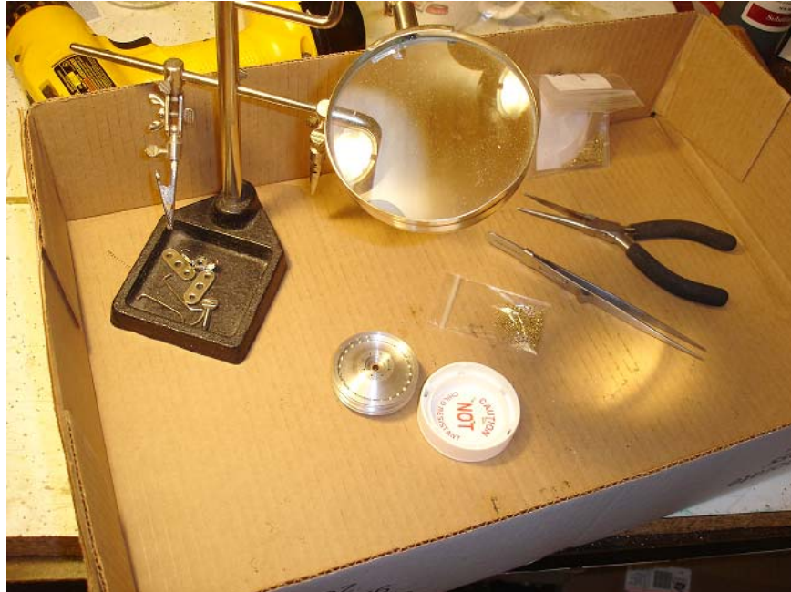
The set up for installing the micro-bolts.
